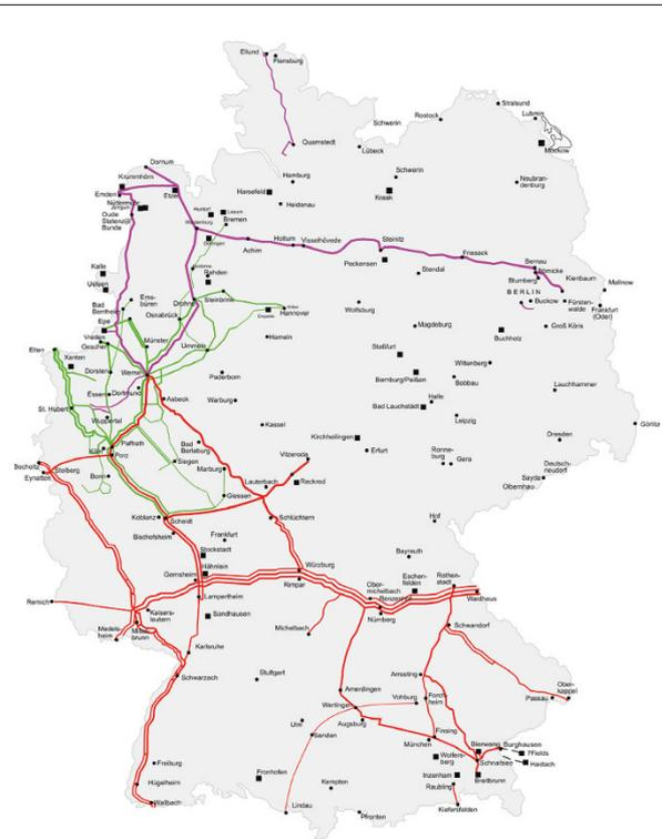
**Figure 1:** The natural gas transport network of Open Grid Europe. The mathematical optimization model for the optimal transport of gas through such a network combines almost all challenges of modern optimization: integer controls, differential equations, highly nonlinear models of physics and engineering, as well as uncertain data.
