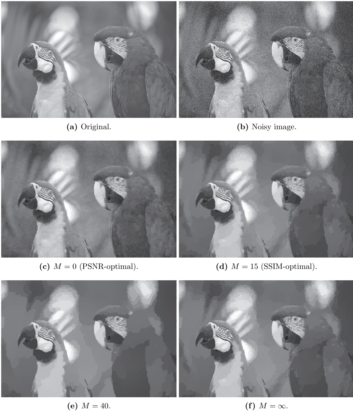
Figure 5. Parrot photo: Denoising results with noise level \sigma = 30 (Gaussian) for varying cut-off M , fixed q = 0.5 , and fixed \alpha^\infty = 0.0253 .
