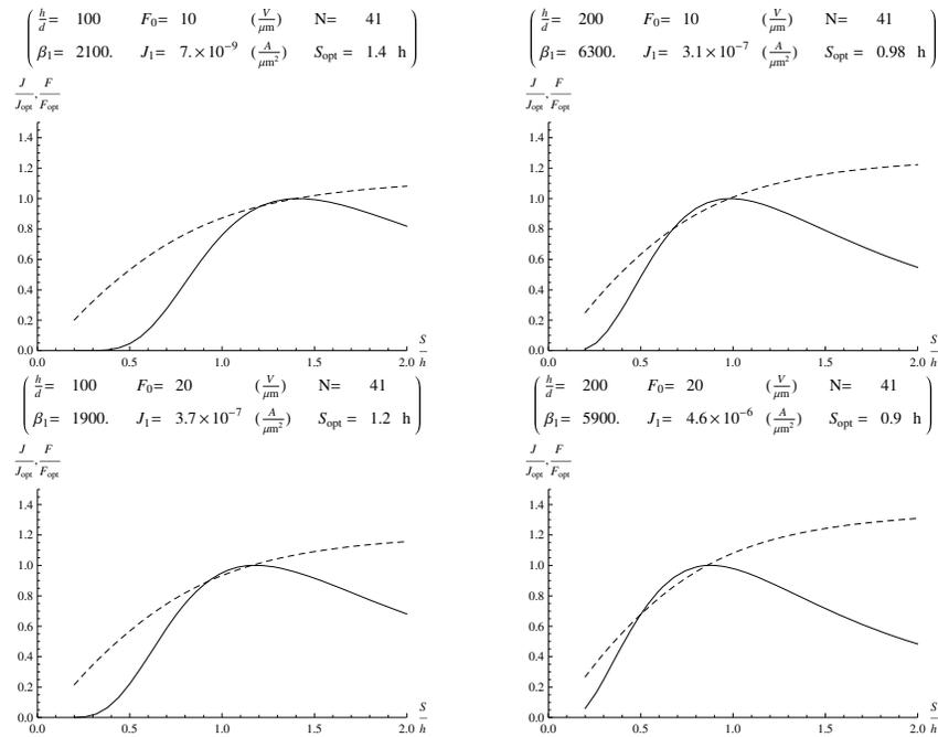
**Fig. 6.** The dependence of field  $F$  and the emission current density  $I$  on the distance between tubes. Both field and current density are normalized with respect to their values  $F_{opt}$  and  $I_{opt}$  for the optimum distance  $s_{opt}$ .
