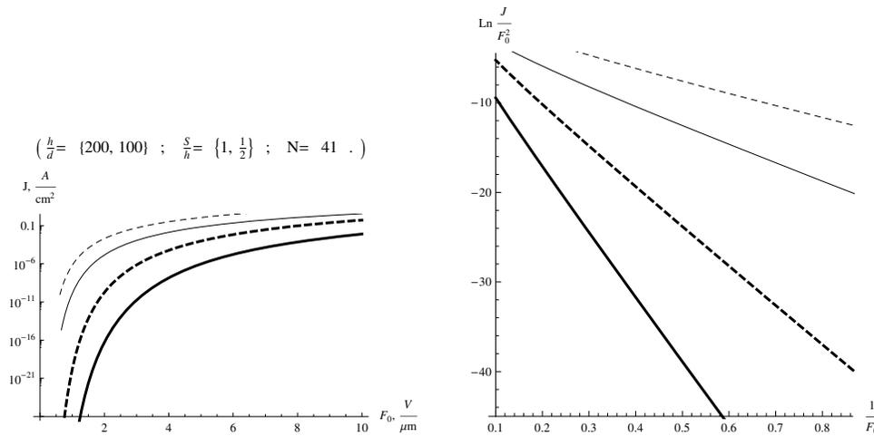
**Fig. 5.** Current–voltage diagram in  $(I, V)$  and  $(\log \frac{I}{V^2}, \frac{1}{V})$  coordinates for the aspect ratio of tubes  $h/d = 100$  (thick) and  $= 200$  (thin) and the distance between tubes  $s/h = 0.5$  (solid) and  $= 1$  (dashed).
