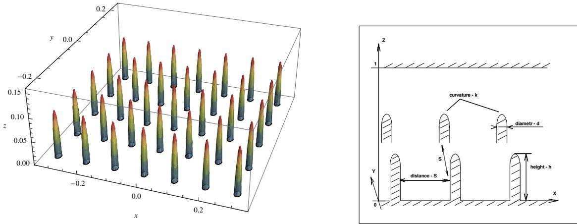
**Fig. 1.** Fast oscillating boundary. The scheme of the regular array of tubes.
