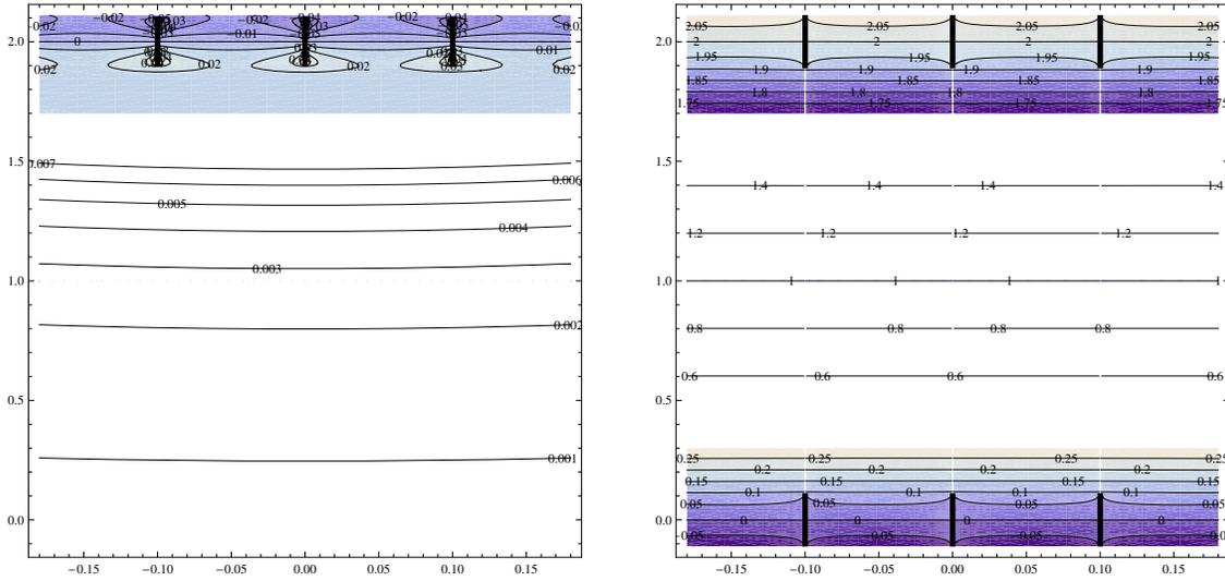
**Fig. 2.** Level curves for the potential  $V_{\text{refl}}$  (left) and for the solution  $u = z - V + V_{\text{refl}}$ . Thick vertical intervals illustrate the localized charges.
