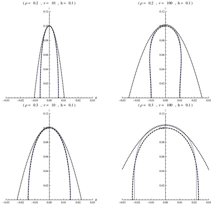
**Fig. 3.** Function  $u$  zero-level surface  $\Gamma$  (solid) and its asymptotics  $\Gamma_0$  (dashed) and  $\Gamma_{top}$  (dotted) for different  $\nu_1$  and  $\nu_3$ .
