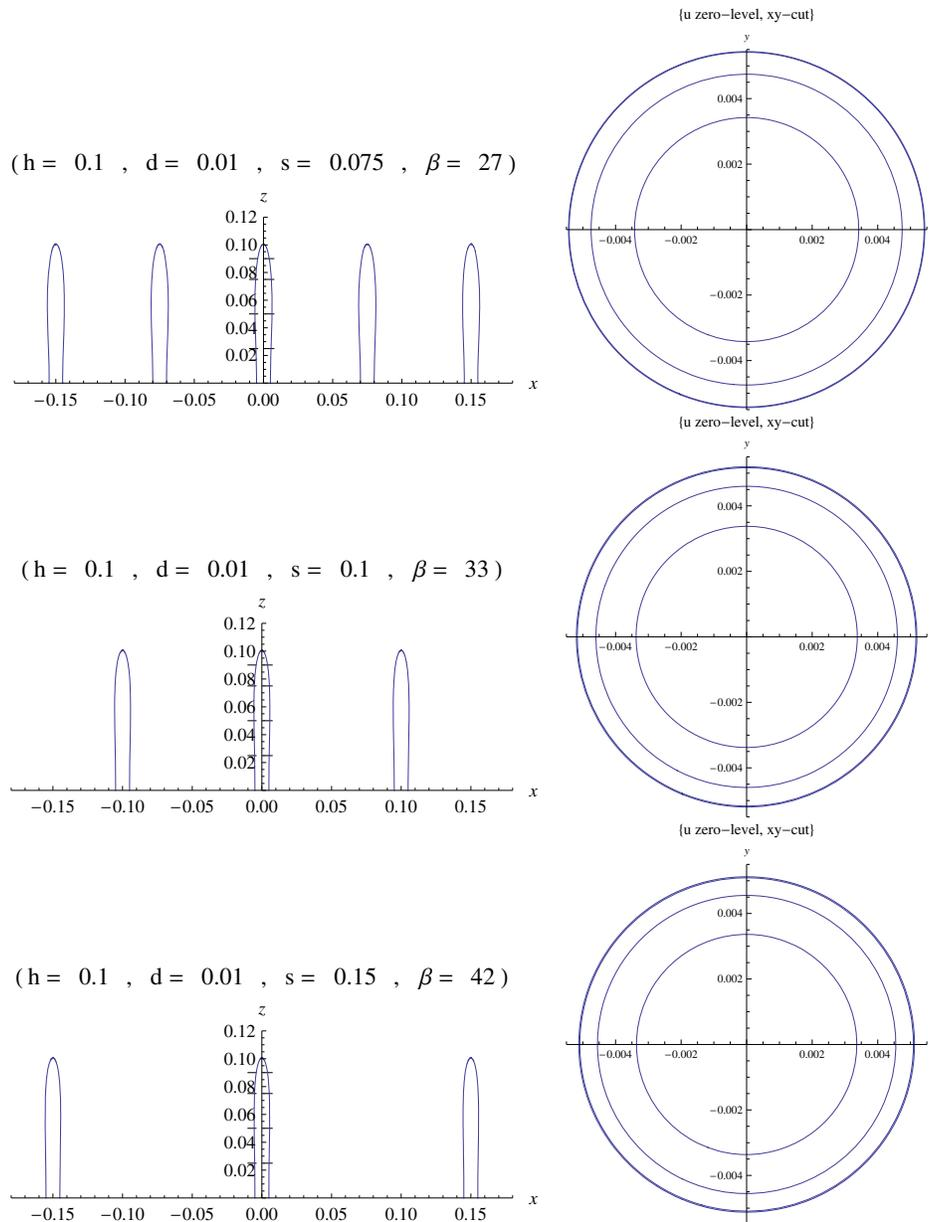
**Fig. 4.** Zero level curves of function  $u$  in the plane  $y = 0$  (left) and in the planes  $z = \text{const}$  (right) for  $z = 0.5h$ ,  $z = 0.75h$ , and  $z = 0.9h$  for different distances  $s$ .
