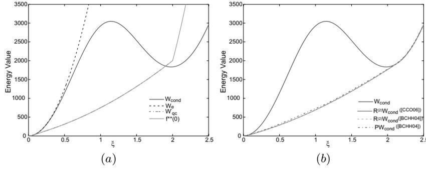
**Fig. 5.2.** (a) Bounds to the quasiconvex envelope of the condensed energy for zero dissipation; (b) Polyconvex and second-order laminate envelope for the condensed energy density in single-slip plasticity.
