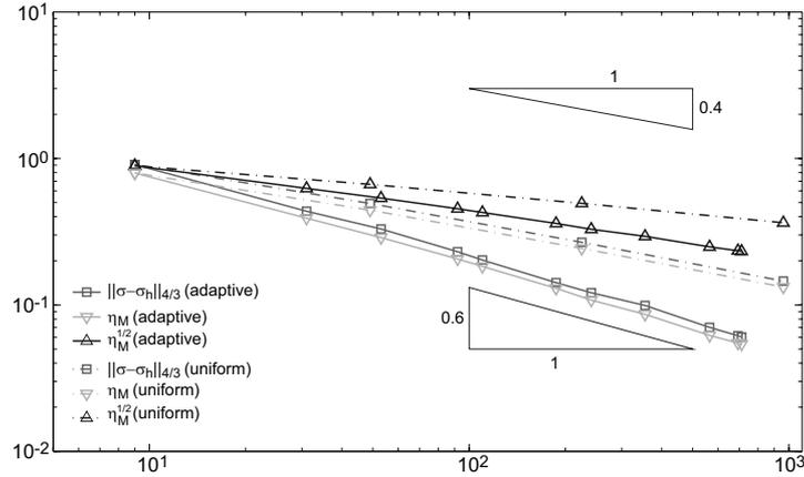
**Fig. 2.1.** The 2D benchmark problem. Experimental convergence rates for  $\|\sigma - \sigma_h\|_{L^{4/3}(\Omega; \mathbb{R}^2)}$  and the error estimators  $\eta_M$  and  $\eta_M^{1/2}$  plotted against degrees of freedom  $N$  with a logarithmic scale for uniform and adaptive mesh refinement.
