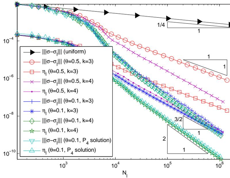
FIGURE 5.4. Convergence history with uniform and adaptive mesh-refinements for the L-shaped benchmark
