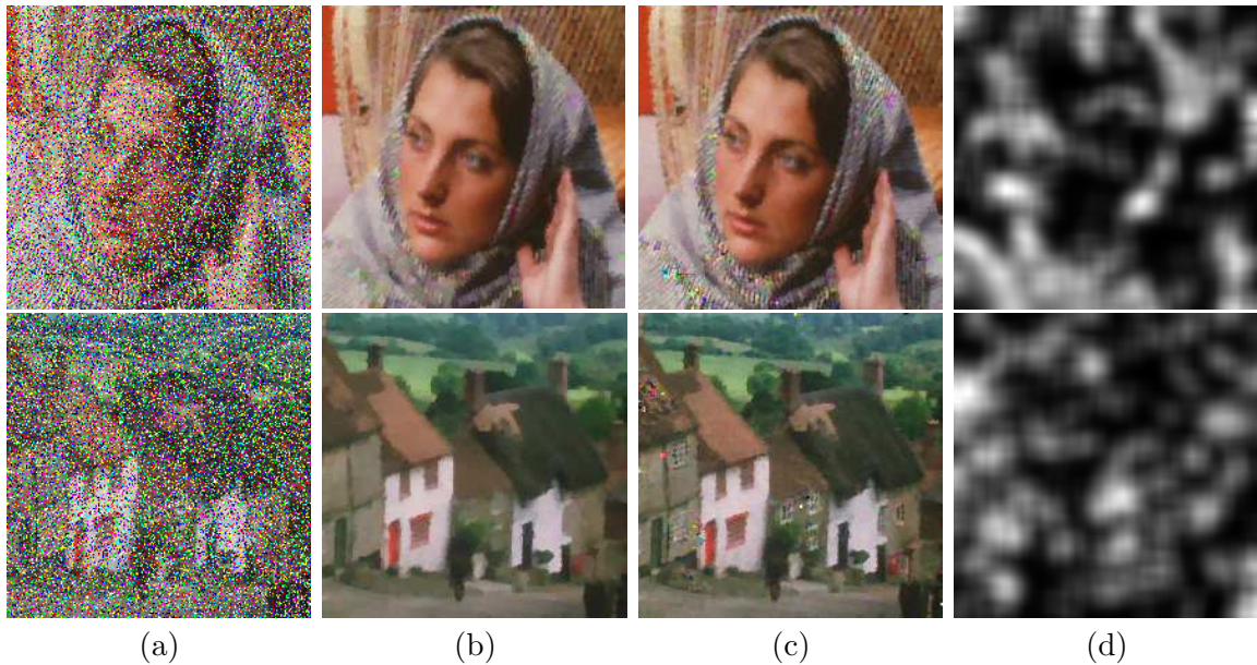
FIGURE 3. Results of removing salt-and-pepper noise for the images “Barbara” (the 1st row) and “Goldhill” (the 2nd row): (a) Noisy images, (b) From VTV-model, (c) From MVTV-model, (d) Final \lambda for MVTV-model.
