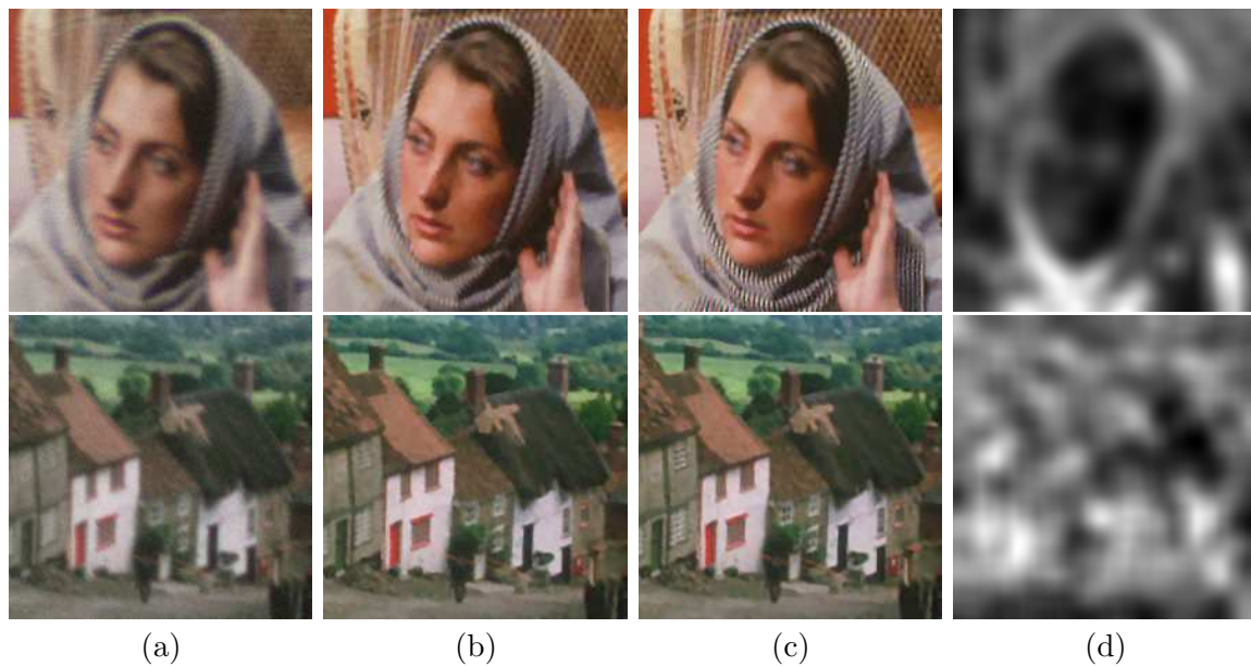
FIGURE 5. Results of restoring the blurred images with Gaussian noise: “Barbara” (the 1st row) and “Goldhill” (the 2nd row): (a) Noisy images, (b) From VTV-model, (c) From MVTV-model, (d) Final \lambda for MVTV-model.
