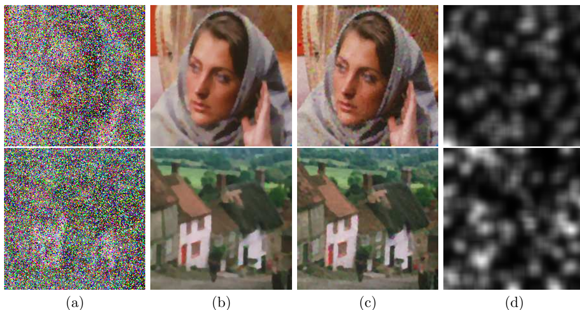
FIGURE 6. Results of restoring the blurred images with salt-and-pepper noise: “Barbara” (the 1st row) and “Goldhill” (the 2nd row): (a) Noisy images, (b) From VTV-model, (c) From MVTV-model, (d) Final \lambda for MVTV-model.
