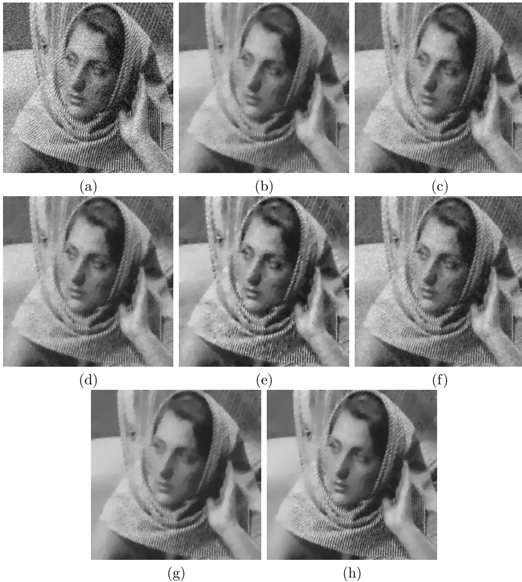
FIGURE 7. Example 1 : Results of different methods when restoring part of the noisy image “Barbara”. (a) Noisy image, (b) TV-method with [10] ( \alpha = 0.088 , PSNR=25.32, MSSIM=0.723), (c) TV-method ( \alpha = 0.06 , PSNR=25.97, MSSIM=0.734), (d) TV-method ( \alpha = 0.07 , PSNR=25.85, MSSIM=0.742), (e) Bregman iteration (PSNR=25.23, MSSIM=0.747), (f) TNV-method (PSNR=25.92, MSSIM=0.716), (g) Basic MTV-algorithm (PSNR=25.43, MSSIM=0.732), (h) Our method (PSNR=26.45, MSSIM=0.785).
